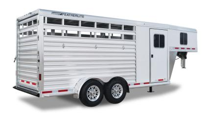
A durable, dependable horse trailer option is the gooseneck Featherlite Model 9751. This slant load gooseneck horse trailer is designed with extruded aluminum sides with air spaces and a full swing rear gate. This model offers an exceptional value with standard features like aluminum wheels and an LED load light.
